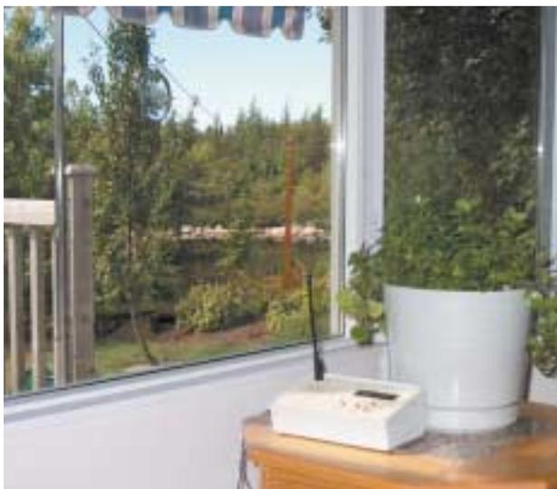
*Photo 1—Here's the actual controller/receiver sitting in my family room. Just visible in the background is a glimpse of the lake—the source of water for the gardens. Not visible is the AC adapter used for power or the power relay, which is located at the electrical panel in the basement.*
