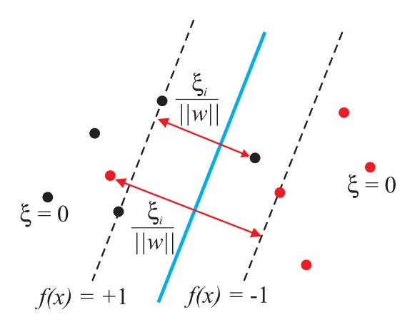
Solution: Regularization, i.e., introduction of slack variables  $\xi \geq 0 \Rightarrow$  Soft Margin SVM.
