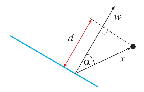
Derivation of the distance d between the observation  $x_i$  and the separating hyperplane  $w^{\mathsf{T}}x_i + b = 0$
