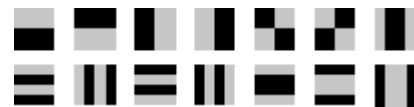
Figure 5. Basic templates of the player. Black areas represent zeros, while gray areas denote value of 1.
