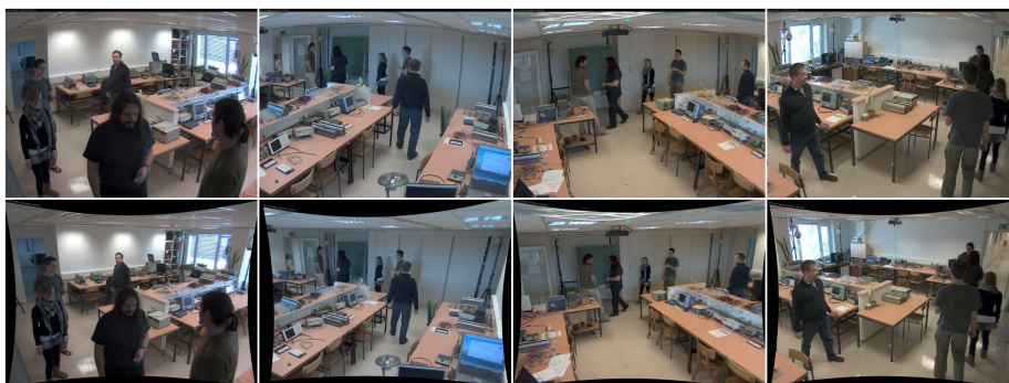
Figure 2: The views from all four cameras. Original images are shown in top row. We use images with lens distortion calibrated and corrected, as shown in the bottom row.
