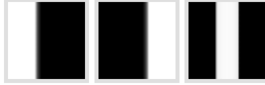
Figure 4. True class template for both pure classes (left, middle) and PV class (right), respectively, plotted as an 8-bit gray-scale image with intensity = 0 corresponding to Q = 0.0 and intensity = 255 to Q = 1.0 .
