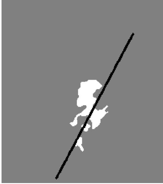
Figure 2. Blob separation. Black line represents pixels that have equal distance to previous positions of both players.
