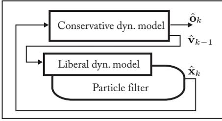
Figure 1: A two-level hierarchical structure of the dynamic model.
