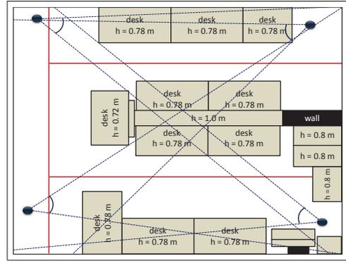
Fig. 1. The experimental setup and cameras’ coverage of room (after lens distortion correction). Red lines mark the paths that the three individuals walked on during the experiment.
